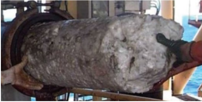
Figure 1 : Hydrate plug extracted from a pipeline [10], [11].
